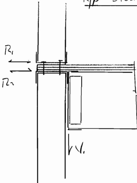
$$\begin{aligned} R_1 &= 159 \text{ lb} \\ R_2 &= 179 / .75 = 239 \text{ lb} \end{aligned} \left. \vphantom{\begin{aligned} R_1 \\ R_2 \end{aligned}} \right\} \text{unfactored}$$
