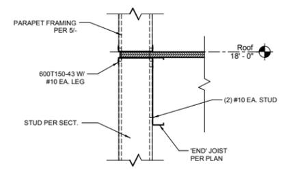
4 ENLARGED SECTION @ ROOF - JOIST PARALLEL
