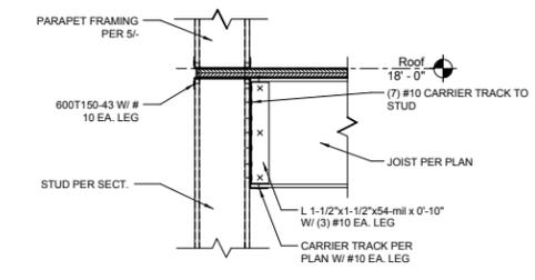
3 ENLARGED SECTION @ ROOF - JOIST PERP.
