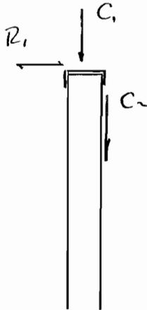
$$C_1 = \underbrace{380}_{\text{roof}} + \underbrace{10.25(20)}_{\text{wall}} = 1085 \text{ lb/stud} \quad [440 \text{ lb LL} + 645 \text{ lb DL}]$$
