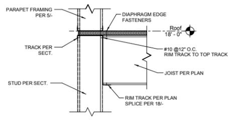
17 ENLARGED SECTION @ ROOF DIAPHRAGM EDGE
